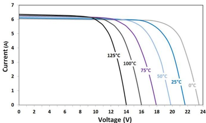
As the cell temperature increases, the voltage produced by the panel decreases. Conversely, as the cell temperature reduces, the voltage increases.
