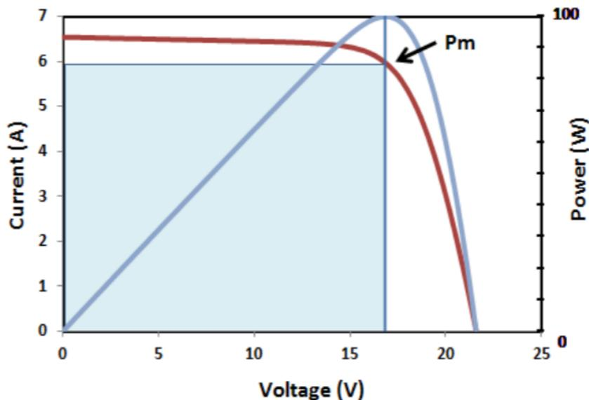
The product  $V_m \times I_m$  is proportional to the area of the rectangle (above). Maximum Power ( $P_m$ ) is reached when the area of this rectangle is at its largest.
