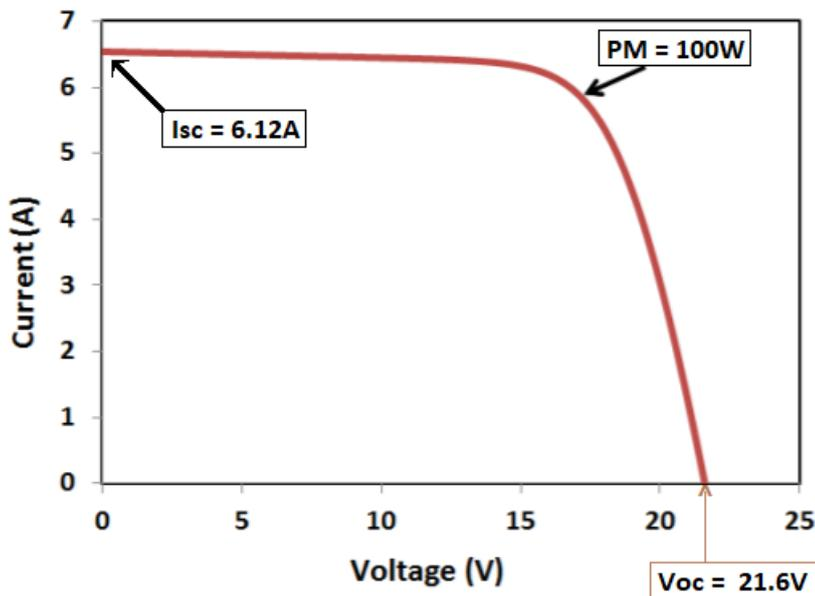
\*Standard Test Conditions (STC)\* are the industry standard for the conditions under which a solar panel is tested. By using a fixed set of conditions, all solar panels can be more accurately compared and rated against each other. The test conditions are defined as follows - irradiation: 1000 W/m<sup>2</sup>, temperature: 25°C, AM: 1,5 (AM stands for Air Mass, the thickness of the atmosphere; at the equator, air mass = 1, in Europe approx. 1,5).
