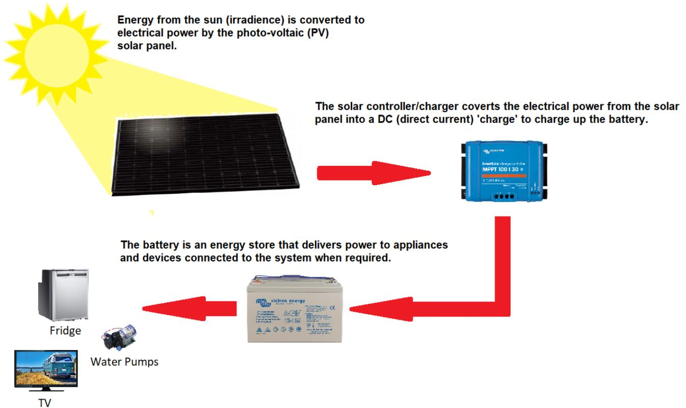
So, a complete system requires a solar panel or panels, a controller/charger, battery and the various fuses, cable and connectors to hook it all together.
