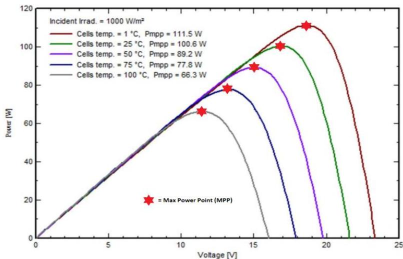
As the voltage changes, the Maximum Power Point (Mpp) moves. The MPPT controller/charger needs to track these changes in order to maintain the optimum charge to the battery.
