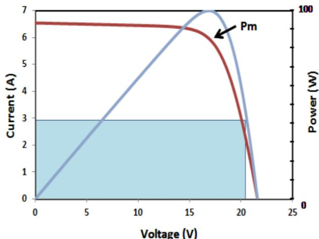
If the voltage is too low (above-left) less power is harvested from the panel. If the voltage is too high (above-right) less power is harvested.
